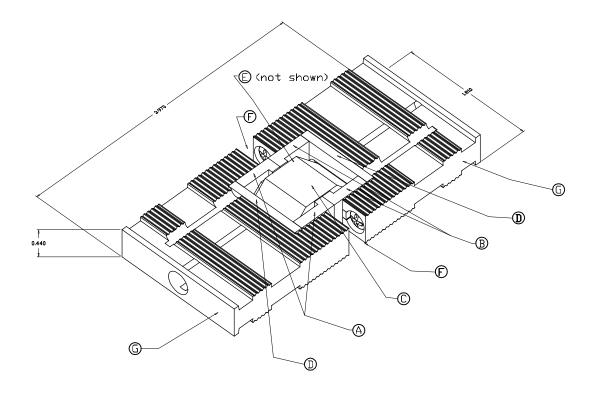
The BFH-4S-200/225K Butt-Fit Hinge Kit consists of the following items:
